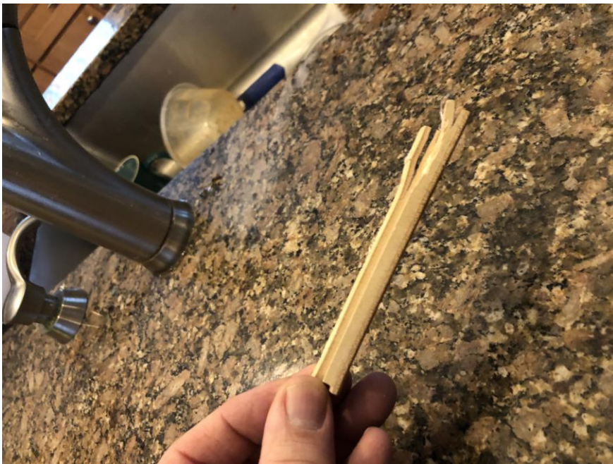
5-Ply Oak engineered flooring, clear grade. There will be a small area of engineered floor that needs replacement. Under 10 square feet.
