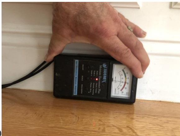
Images 13 & 14 are the master bedroom floor. High moisture content readings and baseboards are popping away from the wall surfaces
