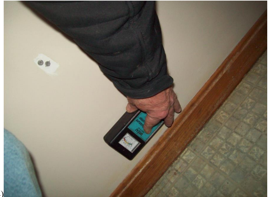
3) Images 3 and 4 are the common wall to the utility area in the employee bathroom– again the moisture meter is at maximum saturation readings
