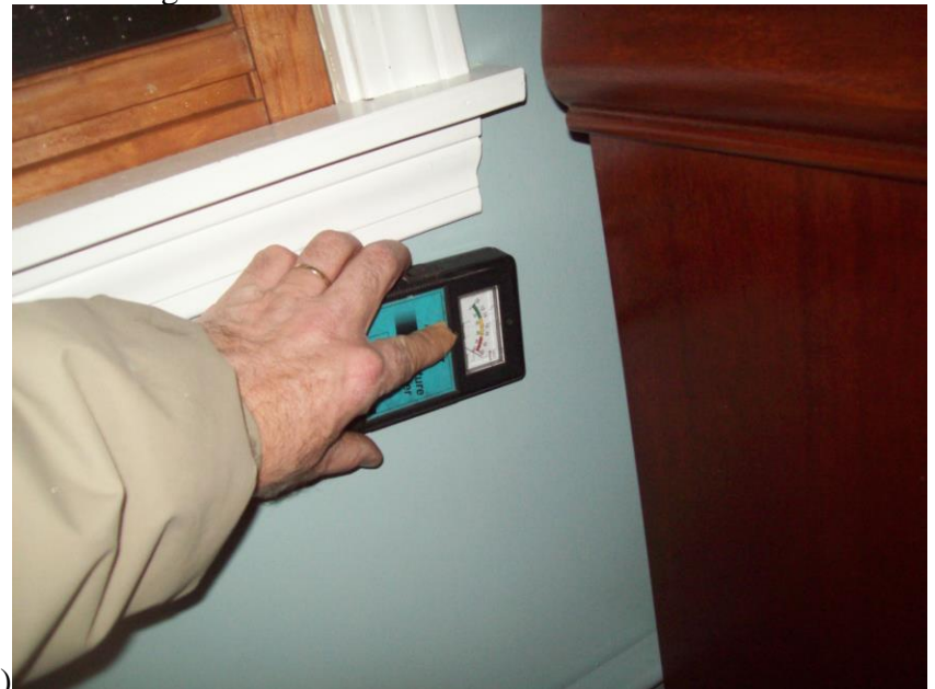
Master bedroom – moisture is likely in a solid state frozen in the wall – moisture meter reading is at maximum
