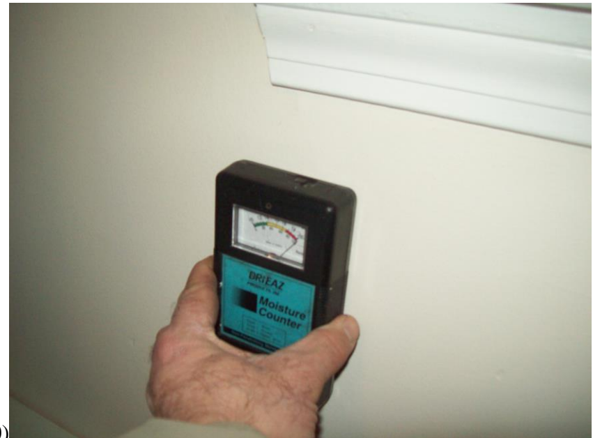
Another second floor bedroom that has very heavy saturation of drywall – again the moisture meter is at maximum level
