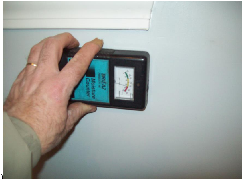
Same bedroom showing very high moisture readings
