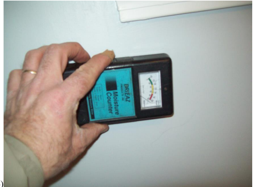
Master Bathroom has extensive water, probably in frozen state and reading at maximum level on the moisture meter
