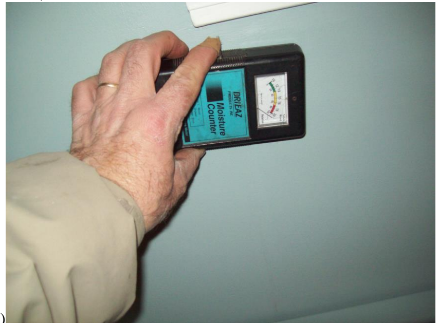
Master bedroom – moisture is likely in a solid state frozen in the wall – moisture meter reading is at maximum
