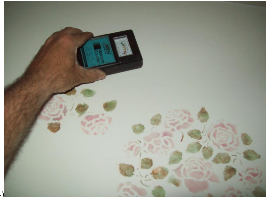
3) Water from the ceiling absorbed in the wall below the toilet and then migrated across the ceiling into the wall common to the staircase.
