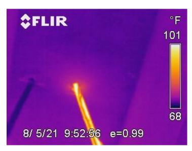
CLIENT REPORTED INSULATION FELL OFF THE UNFINISHED BASEMENT CEILING AND THERE WAS WATER ON BASEMENT FLOOR. THEY COULD NOT PINPOINT THE LEAK. IT TOOK ADVOCATE TWO MINUTES TO DETERMINE IT WAS THE FIRST FLOOR SHOWER MIXING VALVE – NOTE ON THERMAL IMAGE 3 THAT HOT WATER IS RUNNING **OUTSIDE** THE PEX HOT WATER FEED\*\*\*
